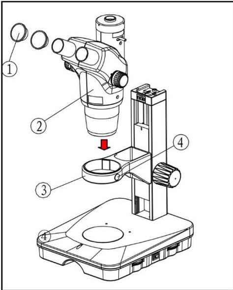
**Fig. 1****Mounting the Trinocular Head (Fig. 1)**
