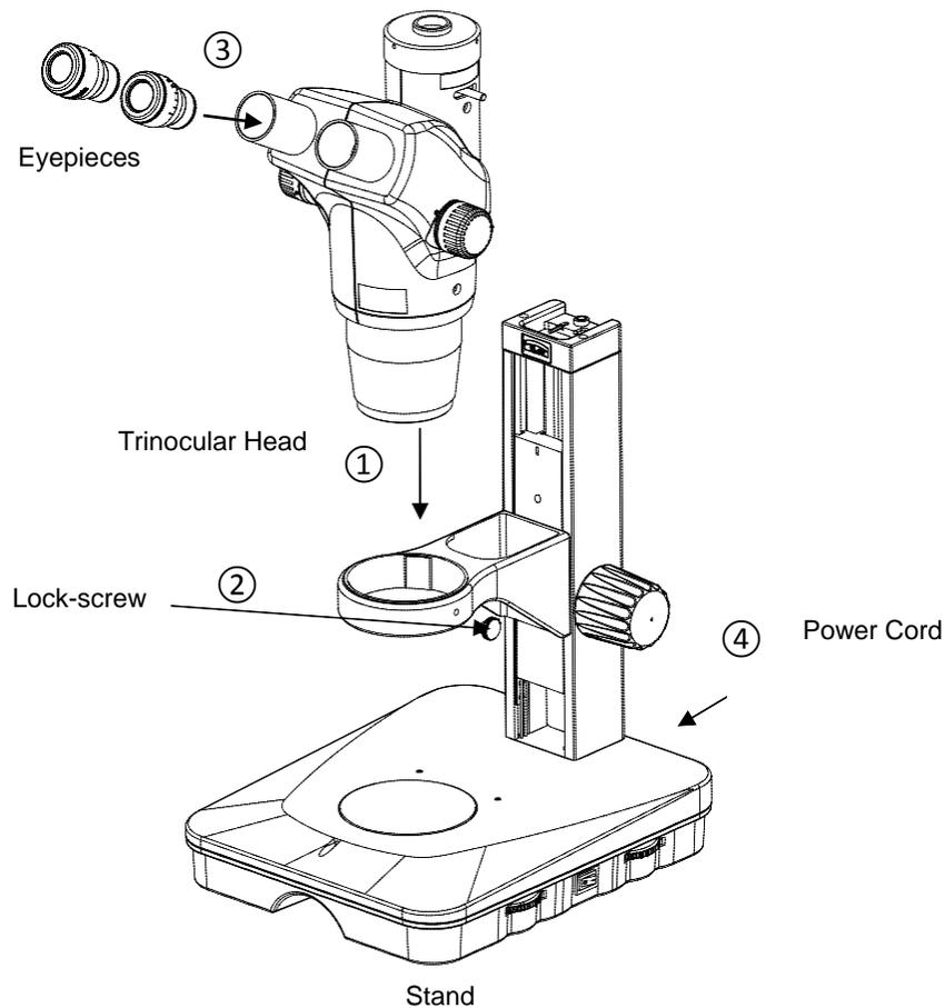
**DETAILED ASSEMBLY PROCEDURE**
