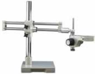
The Dual Boom Ball-Bearing Stand features a 26" stainless steel horizontal boom extension (limited to 24" when used with a System 373 model) and a 17.5" vertical boom mounted to a 10" x 10" die-cast base. Ball-bearing design allows fluid horizontal extension of the boom stand. The focus mount angles to 45° to permit additional viewing and inspection perspectives. For use with all Luxo System 273, 373 and VIP microscopes.
